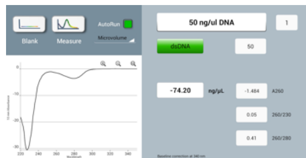
Figure 1: DS-11 Negative spectra obtained due to blanking on a dirty sample surface
